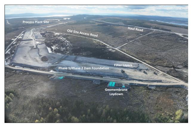
Figure 2: Construction of the Tailings Management Facility, Looking West. October 2023
