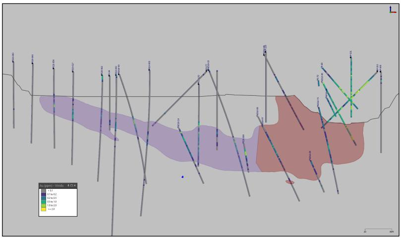
Figure 14-4: Cross-section Looking North along the Northing 14,280,385 N (purple – Banshee domain, red – North Pan domain
