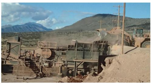
Figure 17-3: 36x50" Lippman Jaw Crusher with Stockpile Loading
