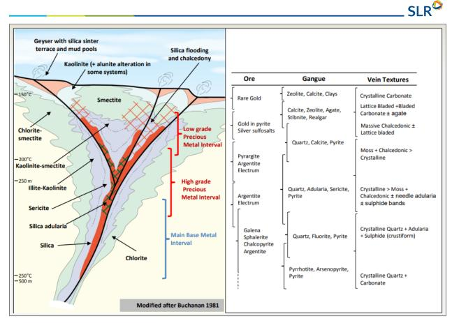
Figure 8-1: Low and Intermediate Sulphidation Epithermal Vein Model
