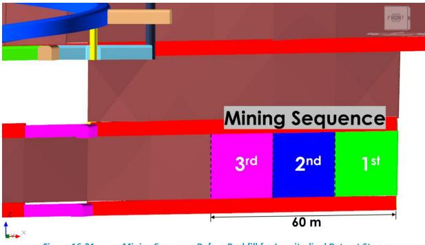
Figure 16-31: Mining Sequence Before Backfill for Longitudinal Retreat Stopes
