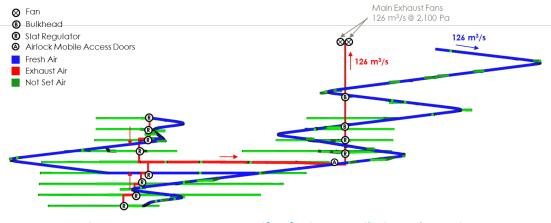
Figure 16-35: Stage 3 – Life of Mine, Ventilation Schematic
