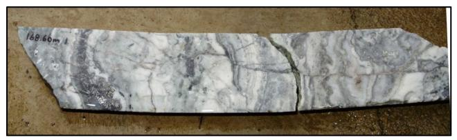
Figure 7-9: Banded Low Sulphidation Epithermal Quartz Vein from Drill Hole RD10-009 (168.60 m). Example of Preserved Primary Textures
