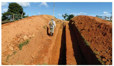
Figure 9-8: Prototypical Exploration Trench - EBP
