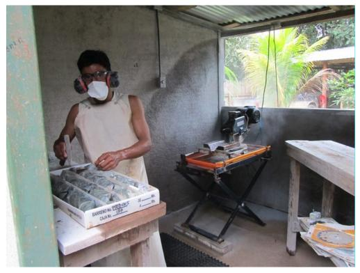
Figure 10-11: Core Cutting Facility
