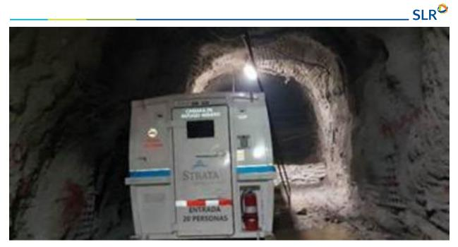
Figure 16-26: Portable Mine-Rescue Refuge Station at Jabalí West UG
