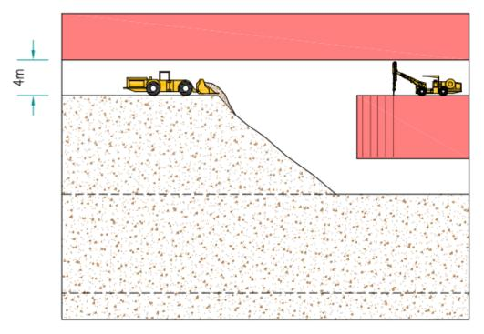
Figure 16-23: Avoca Method – Gap Left between Rock Pile and Bench
