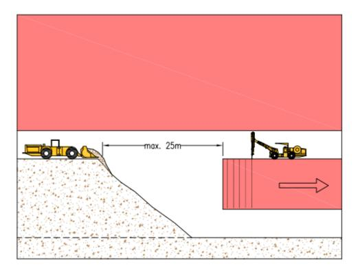
Figure 16-21: Avoca Method – Backfilling
