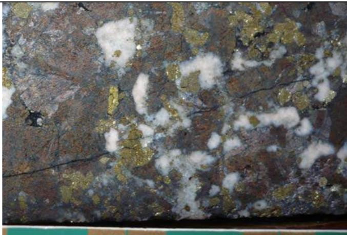
Photo 7: CA08-16 (143.7m; 5.92 g/t Au, 44.8 g/t Ag, 1808 ppm Cu, >10,000 ppm Zn). Patchy sphalerite-chalcopyrite-galena replacement of strongly sericitized (and weakly Kspar altered?) feldspar porphyry.
