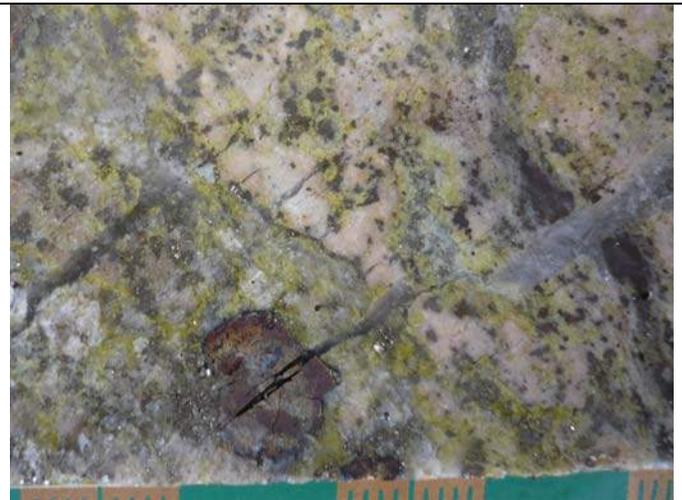
Photo 8: CA08-16 (164.9m; 0.33 g/t Au, 2.8 g/t Ag, 18 ppm Cu, 1698 ppm Zn). Clot of coarse sphalerite associated with silicification in epidote altered calcareous sediment. Note grey anhydrite veinlet.
